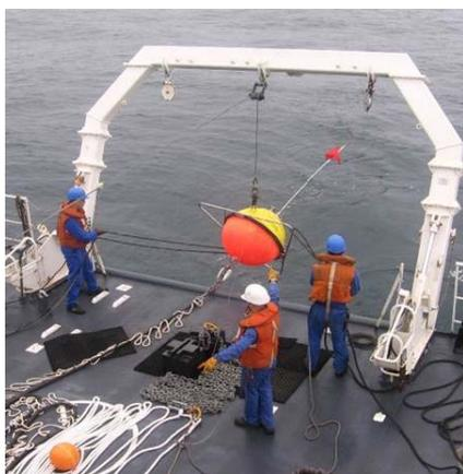
**Figure 14: Waverider buoy with mooring chain and bungee**
